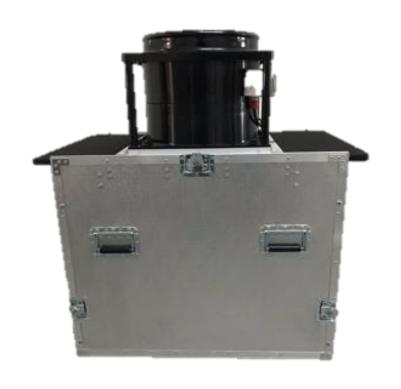
Air Scrubber are use to remove micro particle in the air, such as mold, bacteria, virus etc. With a high powered turbine blower delivering up to 9000 cubic meters of air exchange per hour. This create a cyclone effect forcing air upwards thus creating a downwards draft back toward the machine further enhancing its particle extraction capabilities.
